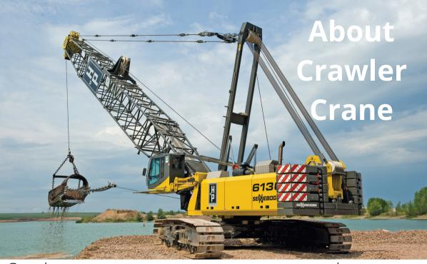
Crawler cranes are cranes mounted on an undercarriage with a set of tracks, or crawlers, that provide stability and mobility. Crawler cranes are used particularly in construction and demolition work, but also in transport for loading and unloading.
