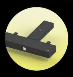
The "T" floor base is constructed of 2"X 4" steel tubing, welded, filled, and damped at the factory. These bases will raise the speaker about 3" off the floor (includes about 1" for the spikes). The "T" base floor bases can be sized match a wide variety of speakers.
